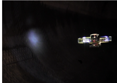
Fig. 1 A quadrotor flying inside a penstock at Allatoona Dam, GA. Lighting is provided by a portable spot light. The quadrotor is equipped with a 1.6 GHz Atom Intel processor, Hokuyo [2] laser scanner and an IMU unit. Note that the installation of lights for illuminating the entire tunnel is impractical. Therefore, we equip our quadrotor with LED lights as shown in the figure.
