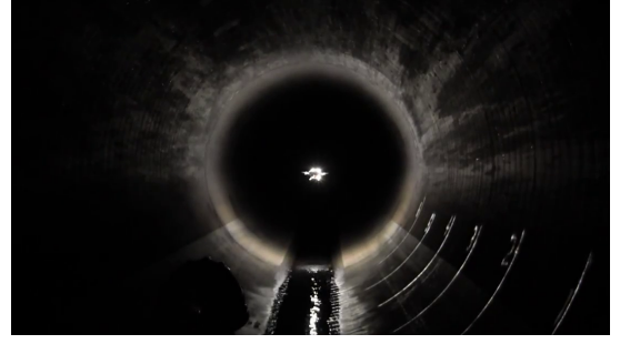
Fig. 10: A snapshot from the experiments inside the Glen Canyon Dam penstock. The robot is flying fully autonomously using on-board illumination. Also in Figure 12 we show the local 3D reconstruction and the 360 degree panoramic image generated using the images from the four cameras.
