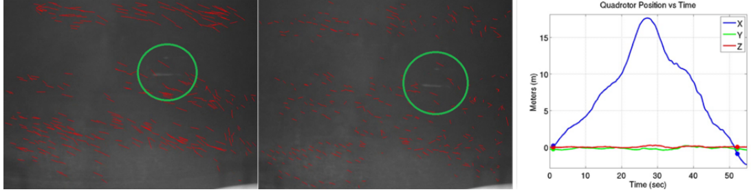
(a) A comparison of axial position estimates at the take off position. We deduce that the robot revisits the same position from the horizontal white scratches circled in green.
