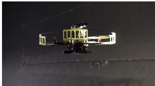
(b) Our Pelican platform flying inside a penstock in Allatoona Dam, GA. In this photo, the robot is also collecting imagery with a uEye camera mounted on top of the lidar.
