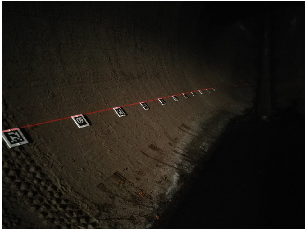
Figure 8.4: ( Top ) The self-leveling laser level is attached at the tunnel surface from its magnetic mount. ( Bottom ) The top edges of the first group of tags are aligned with the laser beam.
