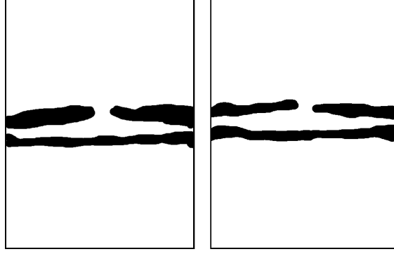
Figure 5.8: Masks applied to the images captured from the right and left cameras. The half strips cover the image areas corresponding to the propellers. When the robot is flying close to the centerline vertically, the side cameras are exposed to specular reflection from the wet tunnel surfaces which degrades the feature extractor and tracker performance. The full strips mask out these image regions.
