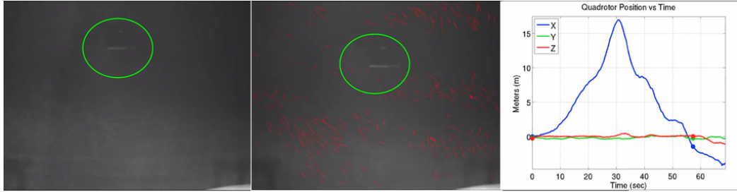
(b) The drift in the axial position after a \sim 40 meters of flight is \sim 2 meters.
