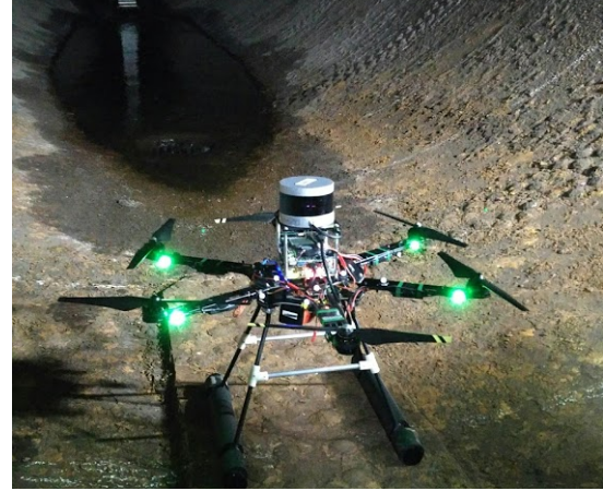
(b) DJI platform with extended arms and E600 propulsion system.
