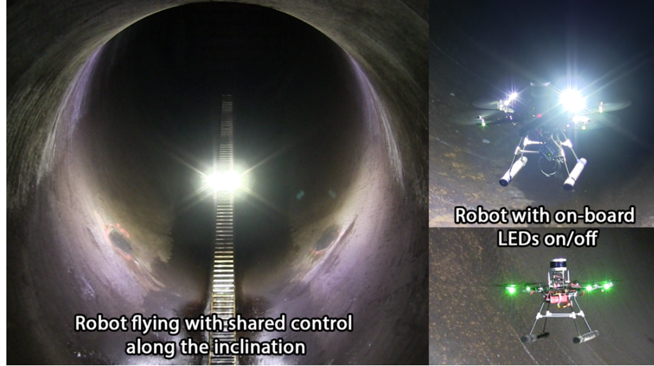
Figure 6.8: Photos of the DJI experiment platform flying inside a penstock at Center Hill Dam, TN. The onboard illumination is required for the testing. However both for safety concerns and for imagery collection, we kept the LEDs on.
